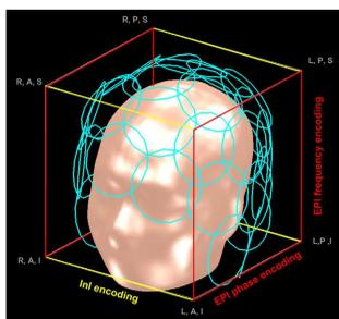
**Fig. 3** EVI: The 3D InI spatial encoding scheme implemented using a high–density 32–channel array of coils.<sup>25</sup>
